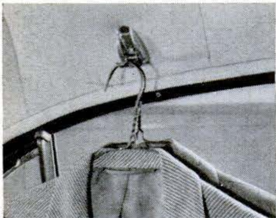
CLOTHES HOOK. Larger than standard garment holders, this one will take up to six hangers of clothes. When not in use, it folds up against the headlining of the car. Pontiac and Kaiser offer it.
